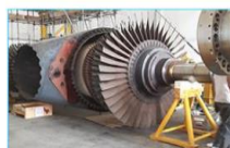
Inner Casing with Turbine Rotor and Inlet Guide Vane(IGV)
