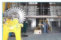
De- Bladed Turbine Rotor Disc
